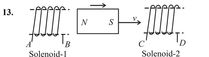
In the above diagram, a strong bar magnet is moving towards solenoid-2 from solenoid-1. The direction of induced current in solenoid-1 and that in solenoid-2, respectively, are through the directions:
